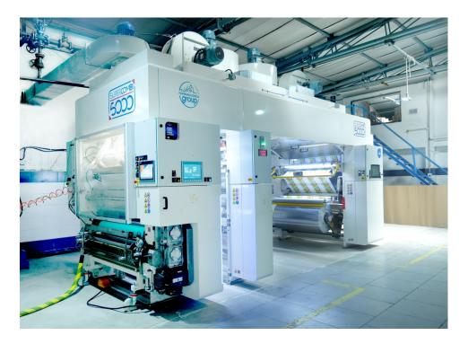
Looking at the growing demand for value added solutions such as HSL coating, water based adhesive lamination, in-register cold seal adhesive and foil-to-foil based lamination, the Company has successfully commissioned its Nordmeccanica Supercombi 5000 laminator.
